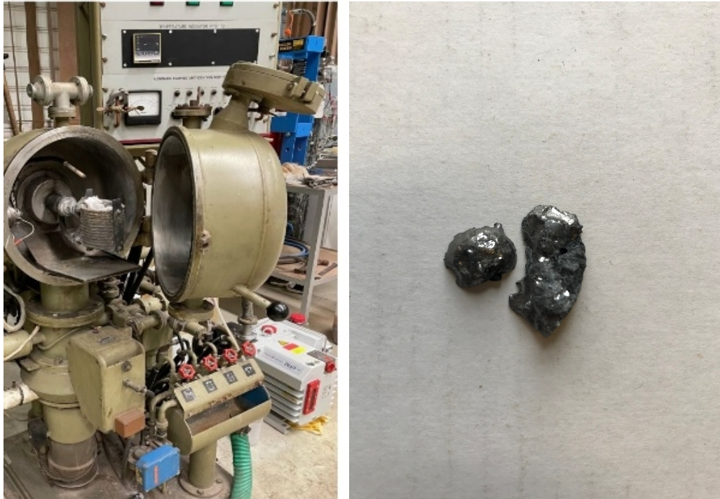
Figure 4. Left: Induction Furnace used in experiments; Right: Ferrotitanium alloy produced.
